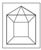
The representation of a body, e.g. a cube with an attached half octahedron, in a 3-dimensional rectangular coordinate system can be done in different ways. In the case of the *single plane projection*, an object is projected onto a drawing plane. The *perpendicular projection* onto the *x*-*y*-plane in a coordinate system is usually called the *ground plan*, the projection onto the *y*-*z*-plane is called the *elevation*, and the projection onto the *x*-*z*-plane is
