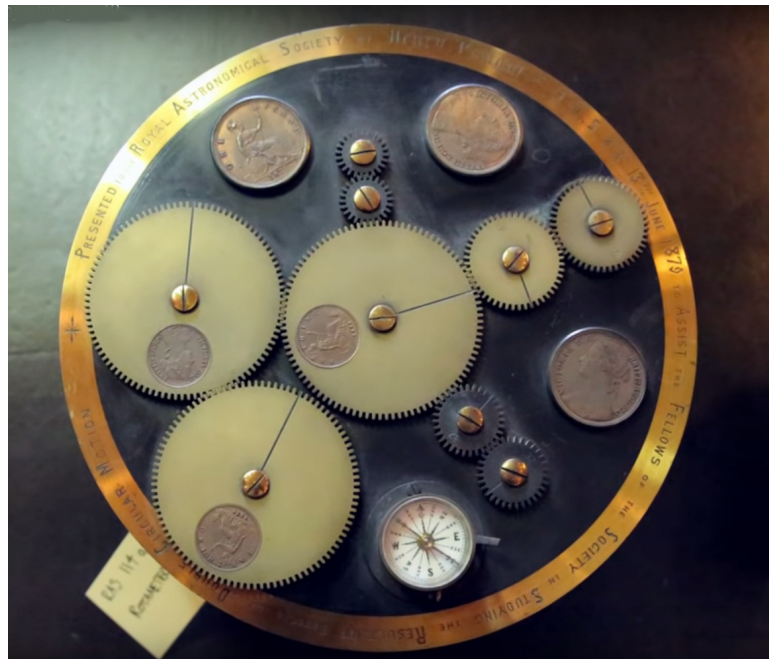
FIGURE 9. One of Perigal's rotameters. The inscription around the rim reads: Presented to the Royal Astronomical Society by Henry Perigal F.R.A.S &c, &c. 13th June 1879 to assist the Fellows of the Society in studying the resultant effects of double circular motion. Photograph courtesy of Brady Haran.
